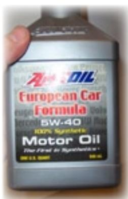
The multi-viscosity, fully synthetic motor oil we chose to use is made by AmzOil®. Any other reputable brand is acceptable. Note that Fox recommends damper oil. Damper oil is OK, but does not stick to the parts as well as the multi-viscosity synthetic motor oil.
