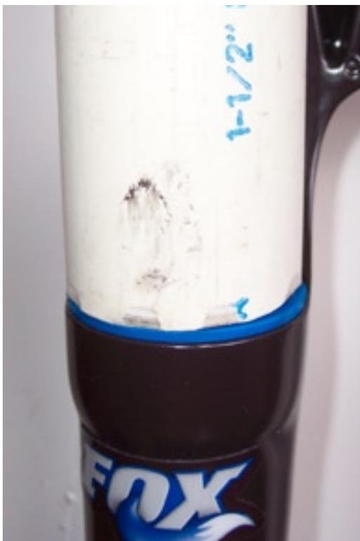
27) Use a large socket or piece of pipe that fits squarely on the shoulder/ flange of the wiper to push the wiper into the seal head. It should start by hand and press most of the way in as you apply body weight to the socket. If the wiper does not fully seal, put some padding under the lowers and
