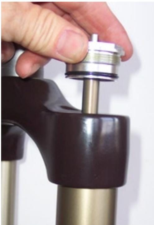
16) Lift up on the damper to speed up the oil draining process. Because this fork uses a sealed damper, you are not actually draining any damping oil during this seal change procedure. The oil being drained is “semi-bath” oil which is used primarily for lubricating the bushing and stanchion interfaces.
