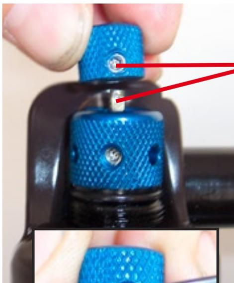
43) Align the low speed compression knob with its respective flat spot on the rod and tighten it down to 4 INCH pounds.
