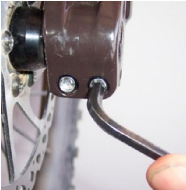
50) Staying on the left leg only, alternate between the two pinch bolts and torque them to 19 INCH pounds.
