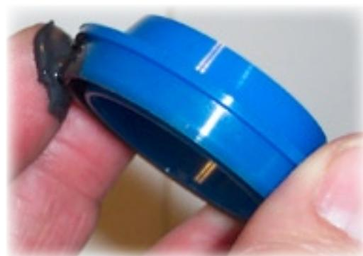
26) Lube the insertion area of the wiper and start it into the seal head by hand.
