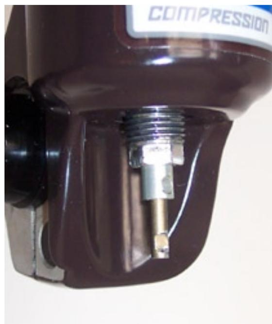
38) Thread the damper top cap into the crown by hand (don't tighten yet).
