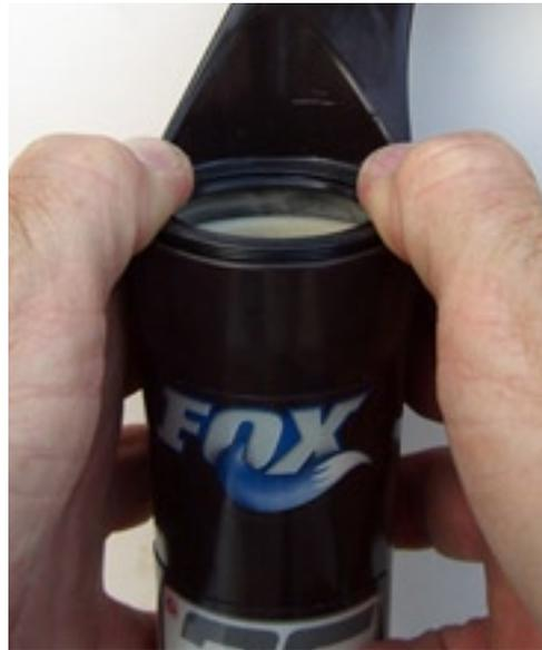
25) Use the back (flat) side of a large socket that closely matches the outside diameter of the oil seal. Press the seal down until it stops against the "step" inside the seal head. Don't push too hard...
