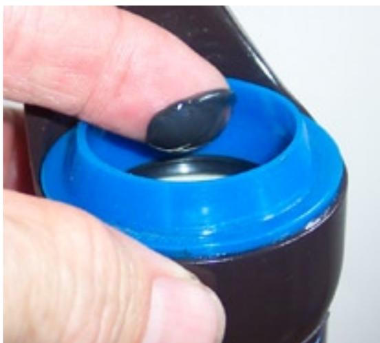
28) Coat the concave areas inside of the oil seals and wipers with Super Slick Grease.
