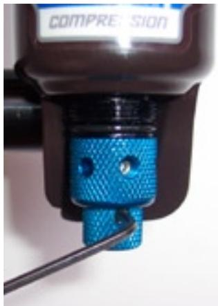
9) Use the 2mm hex wrench to loosen the set screw on the low speed compression knob.
