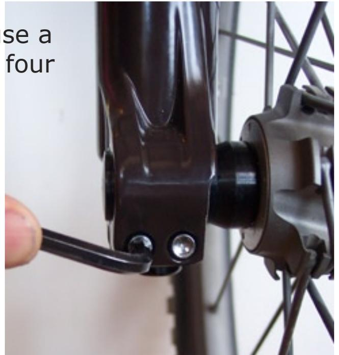
2) Use the same 5mm wrench to turn the 20mm thru-axle counter clockwise.
