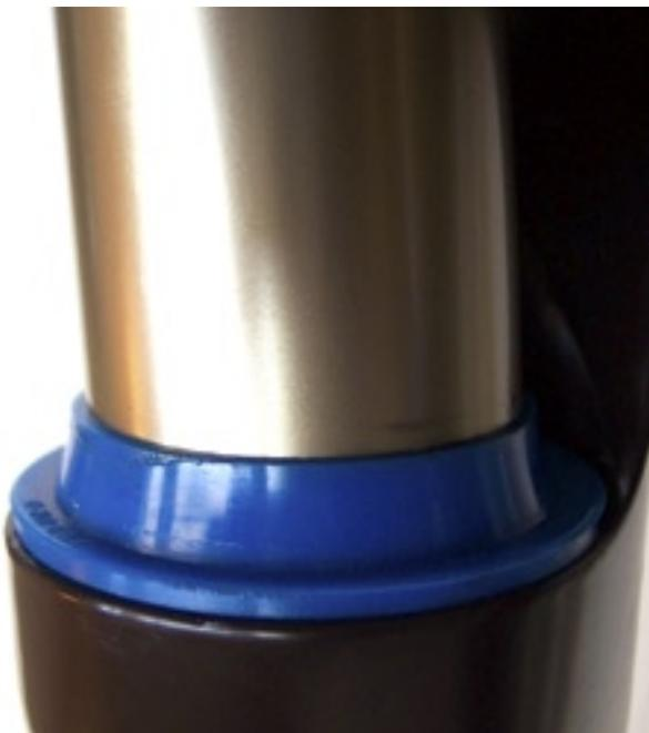
Carefully work one wiper over its respective stanchion tube, then start the other wiper onto its stanchion. **BE PATIENT.** Getting both wipers started may take a few tries. If you force the process, you may damage the wipers or seals. Once the wipers are started evenly, carefully work the lowers up until the stanchions pass the seals and the bushings. **DO NOT SLIDE THE LOWERS ALL THE WAY UP AT THIS TIME.**
