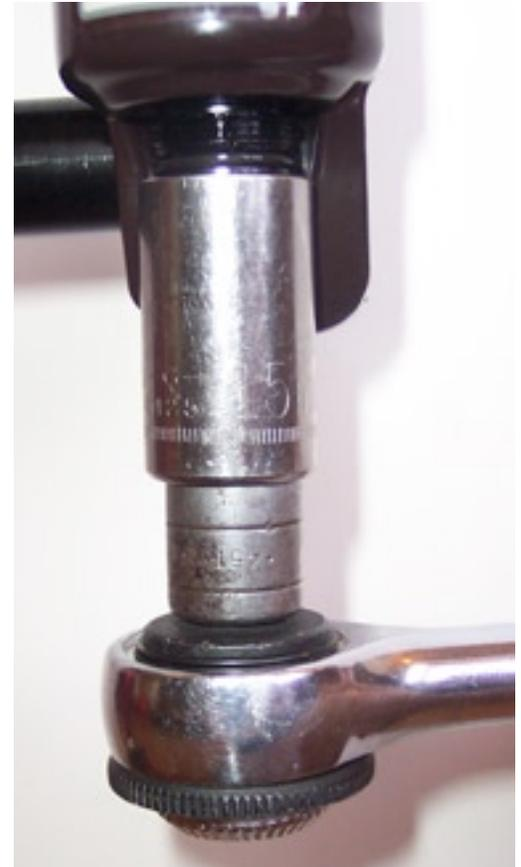
12) With the rebound knob adjusted to about mid-range, hold the knob securely and remove the set screw. Set the knob aside.
