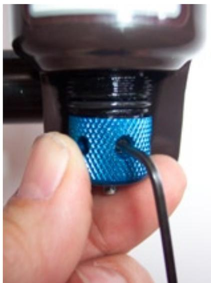
Note the detent ball located in the top of the knob. There is a spring under this ball. Take care not to lose these items!
