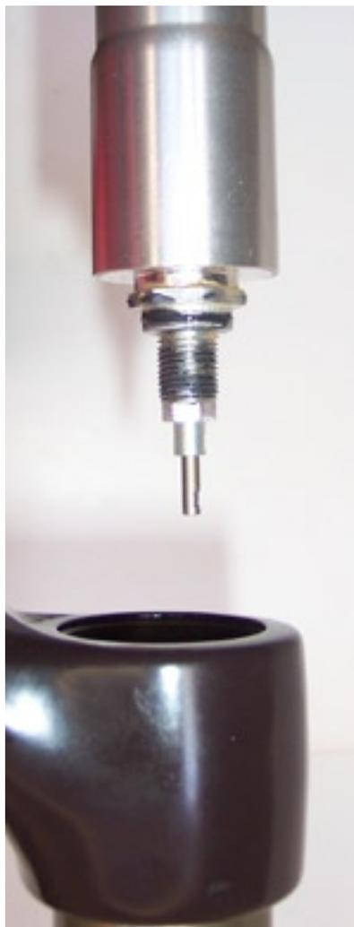
37) Invert the fork and insert the damper through the crown.
