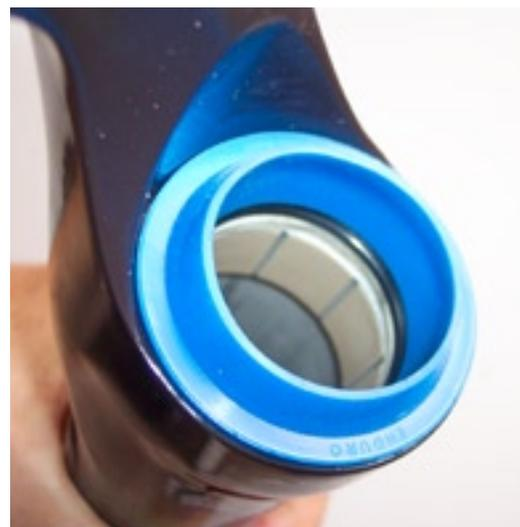
use a rubber mallet to tap the wiper down (Be sure to properly pad the bottom of the leg casting).
