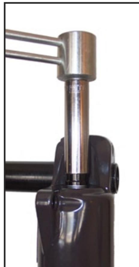
36) Grease the threads and O-rings on the RC2 damper.
