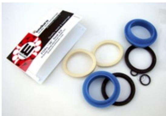
21) Open up the new seal kit and pre-soak the foam rings with oil.
