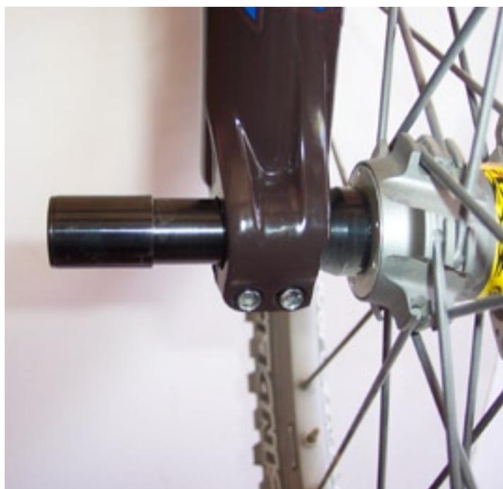
48) Hold the front wheel in place and insert the thru-axle. Start the threads by hand.
