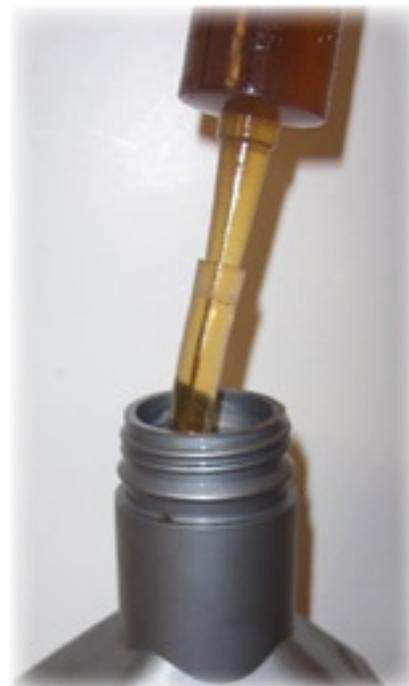
Use a plastic extension tube to draw the oil out of the bottle. Then, remove the tube to inject the oil. (The MixMizer syringe pictured here includes this extension and can be purchased directly at [enduroforkseals.com](http://enduroforkseals.com).)
