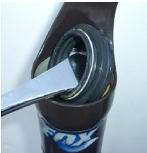
18) Place the lever firmly under the wiper and apply downward pressure on the handle to “pop” the wiper/seal out.
