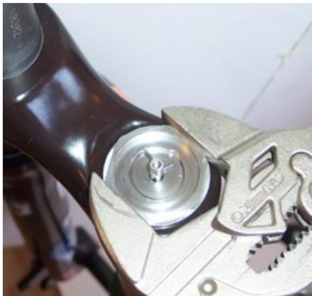
13) Using a good quality adjustable wrench, loosen the damper top cap.
