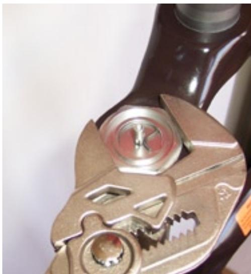
46) Replace the rebound knob and tighten the set screw down.
