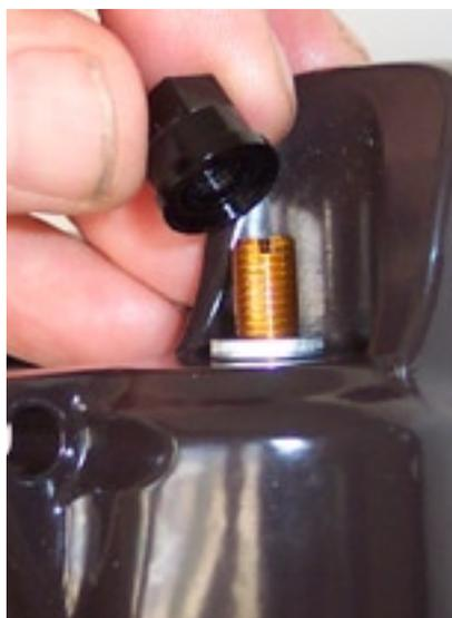
34) Place a new aluminum crush washer over the threaded rod, grease the threads, and hand thread the foot nut.
