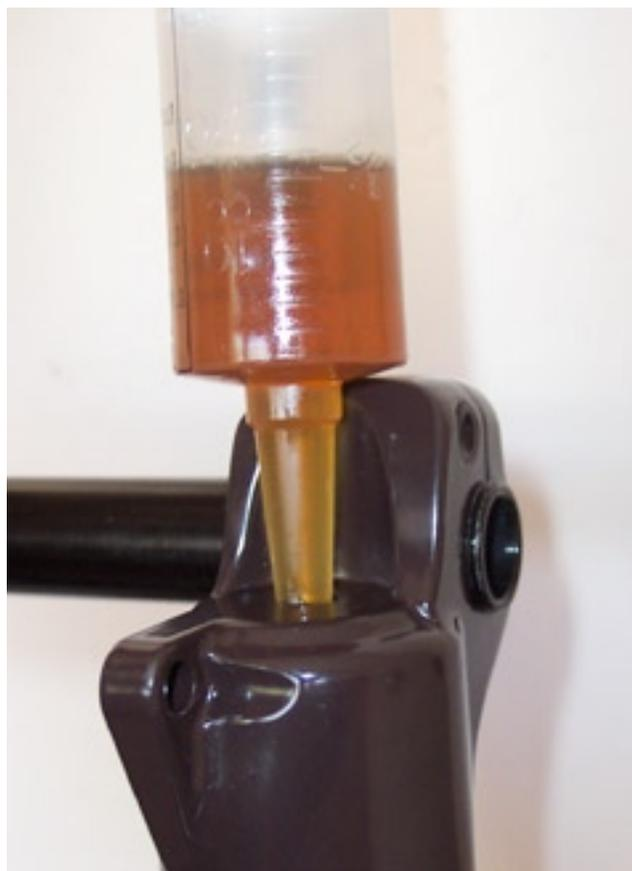
When injecting the oil, don't push the end of the syringe fully into the casting hole. Rather, leave a small gap so the displaced air can escape as the oil goes in.
