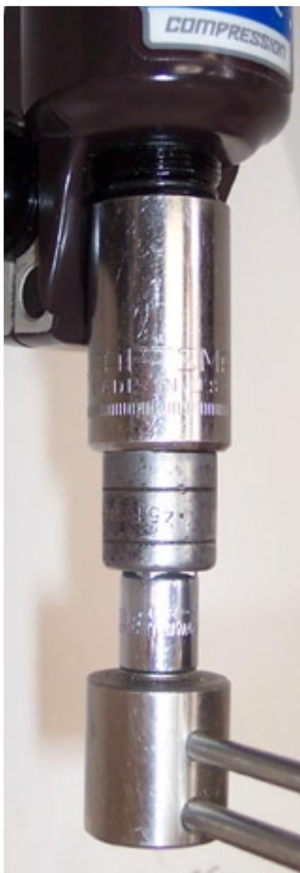
40) Use a 15mm deep socket to tighten the foot nut to about 50 INCH pounds.
