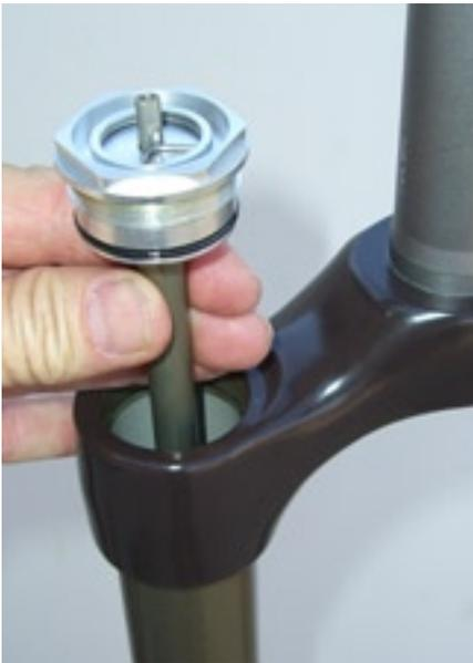
29) Turning back to the upper assembly, pull the damper up through the stanchion tube and set it aside.
