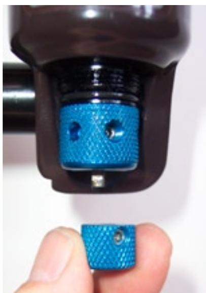
After backing it out a couple of turns, pull the knob straight down to remove it. Note that the set screw tightens onto a specific flat spot on the shaft.
