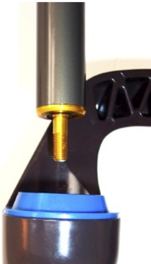
We will now put the upper and lower assemblies back together. By design, we have done nothing with the TALAS leg, which will be extending out of the left stanchion tube. be sure it gets started into the LEFT side of the lower assembly!
