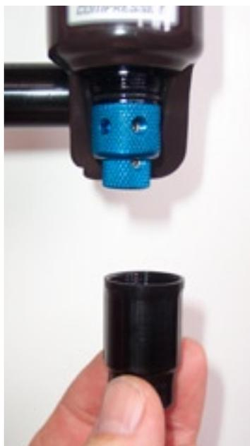
7) Remove the protective cap from the bottom of the damper leg.
