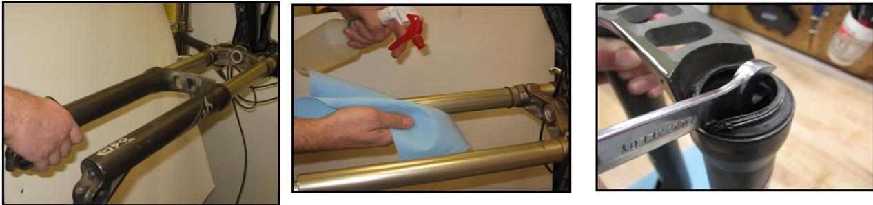
4. Remove foam rings from the lowers. Inspect foam rings for damage.
