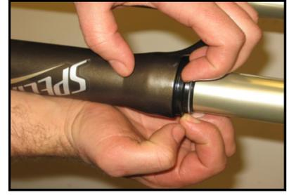
8. Slide lower to top of stanchions. Drop Damper cartridge on the drive side and the Air Spring cartridge on the non-drive. With the cartridge tips exposed at the bottom, torque 60 in-lbs, 6.8 N\*m closed nut and washer onto Damper cartridge. Torque 60 in-lbs, 6.8 N\*m exposed nut and washer onto Air Spring Cartridge. Use a syringe or a beaker and pour 20cc's of 10wt. oil into each fork leg from the exposed top.
