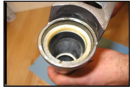
6. Make sure both of the saturated foam rings are sitting in the groove right above the upper bushings. Replace the clean dust wiper seals onto the lowers. Cautiously use a broad surface Allen key or punch to seat seals evenly. Carefully slide stanchions into the lowers, make sure the foam rings and dust wipers do not get hung up on the stanchions.
