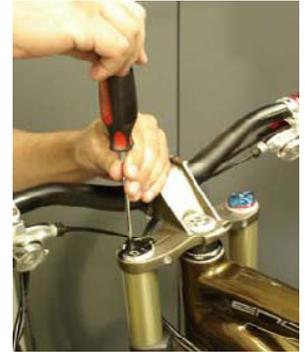
2. Place a Shallow Used Oil collection pan beneath fork. Remove the air cap from the Air Spring Cartridge.
