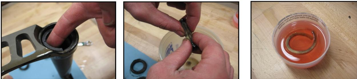
5. Using alcohol and lint free towels, carefully clean the areas where the dust seal and foam rings sit in the fork lowers.
