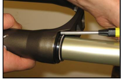
7. If you are using a foam ring that is not split. First slide the clean dust wipers onto the stanchions, then slide on foam rings. Slowly slide the stanchions into the lowers, seat the foam rings and dust wipers. Carefully use a broad surface Allen key or punch to seat the dust wipers.
