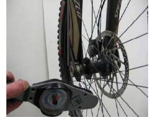
10. Check alignment of stanchion tubes. Loosen and realign if necessary, lightly re-torque crown pinch bolts.
