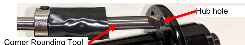
Rounded hole of classic flange hub:
