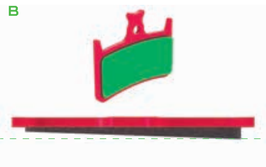
FIG B: A pad worn on a taper lengthwise is evidence of a badly aligned caliper.
