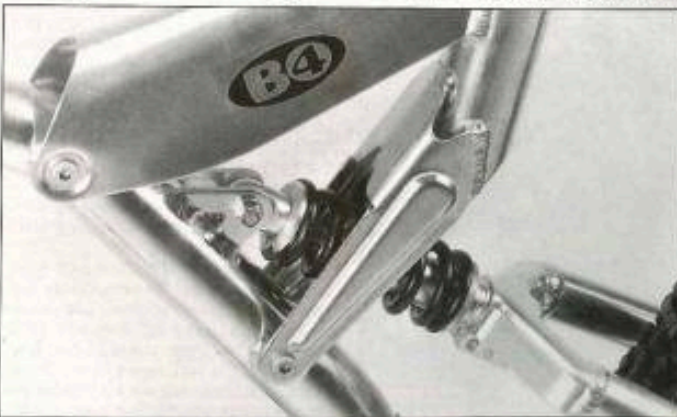
Construction zone: The B-4's interrupted-seat-tube section employs monocoque, CNC machining, formed tubing, bolting and TIG-welded construction—all within one square foot. Minor ride height adjustments can be made by shimming the AMP's shock above its clamped, seat stay crown.
