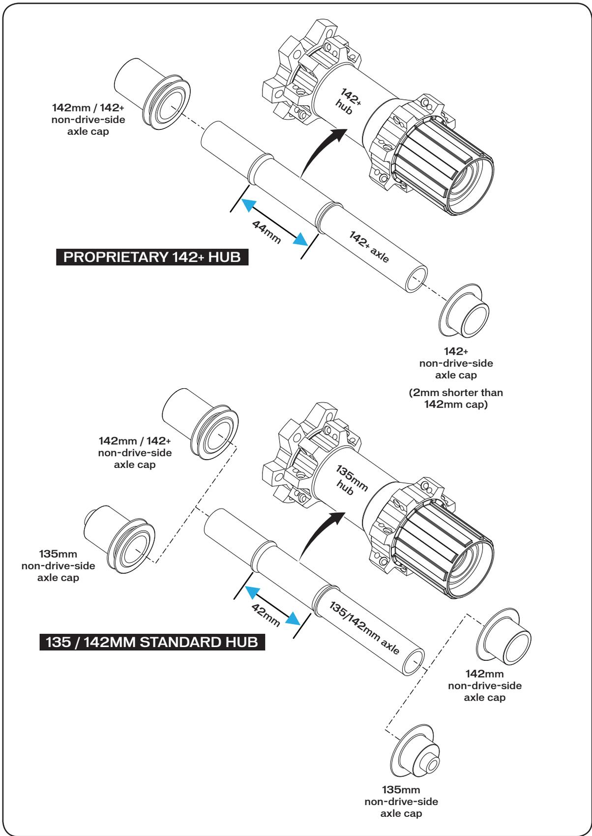
**CONVERTING 135MM HUBS TO STANDARD 142MM**
