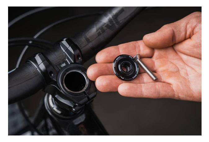
Use the supplied M6 Bolt and Washer and either a hollow cassette tool Park FR 5-2 or 1/4" drive 15mm Socket to pull out the centre portion of your star nut.
