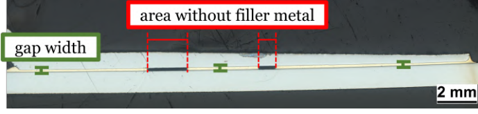
Figure 7: Metallurgical analysis of brazing joints
